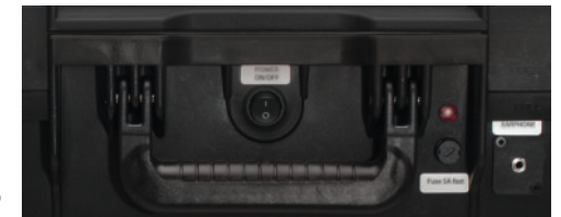
(Image 21) LED & fuse on the front of a case for ATEM Extreme
