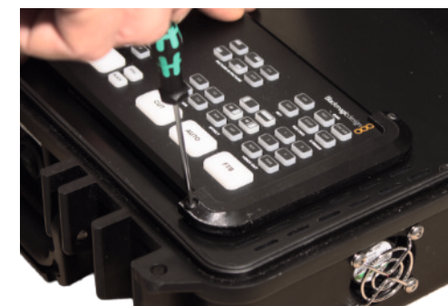
(Image 14) Screw ATEM Mini with C-clamps
