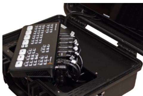
(Image 12) Plug the cable into the ATEM
