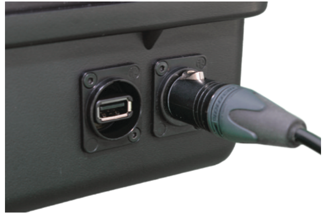
Case with inserted battery connector (XLR 4-pin female version)
