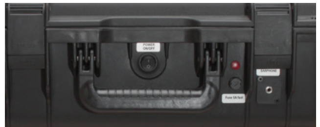
LED & battery power fuse on the front of a case for ATEM Extreme
