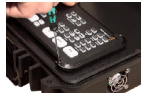
(Image 14) Screw ATEM Mini with C-clamps
