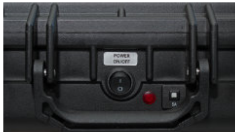
(Image 21) LED & fuse for the battery supply on the front
