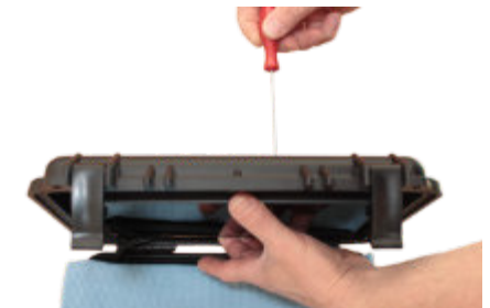
(Image 10) Screw on the monitor
