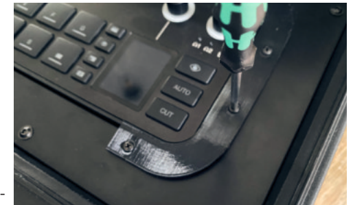
(Fig. 15) Screw C-clamps into the ATEM Extreme G2 case
