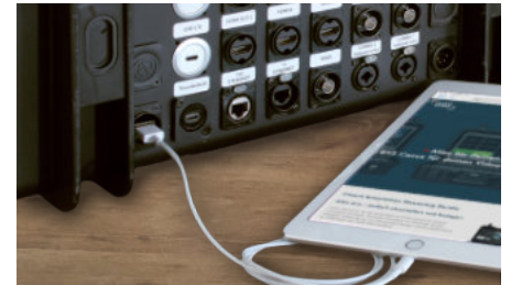
(Fig. 23) USB charging socket with device to be charged plugged in
