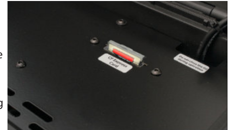
(Fig. 22) Cfexpress card in the mounting slot on the top plate of the BSS case
