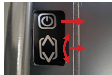
(Fig. 20) Access to the controls on the left side of the monitor
