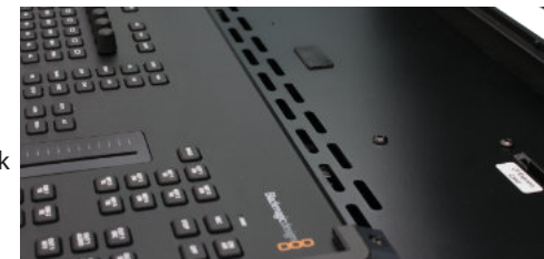
(Fig. 19) BSS case ventilation slots
