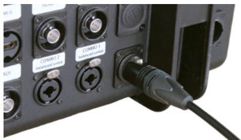
(Fig. 24) BSS case battery connection with attached adapter cable
