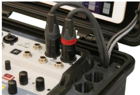
(Fig. 15) XLR plug and cable plugged into Flow 8 Main Out
