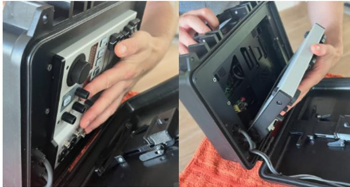
(Fig. 5) Remove the Flow 8; tip the case onto a soft surface and hold the Flow 8 with one hand to prevent it from tipping out
