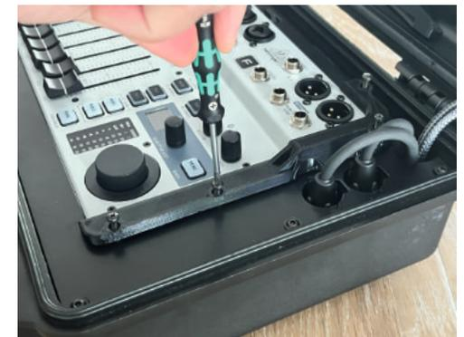
(Fig. 4) Flow 8 Screw down clamp
