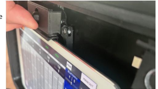
(Fig. 7) Adjust the upper holder to the correct distance and apply the pressure piece
