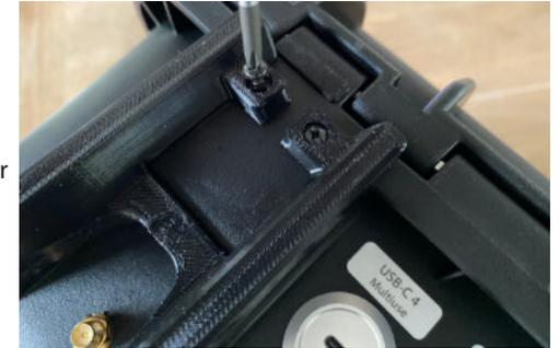
(Fig. 19) Secure the antenna protection with screws
