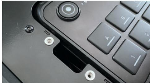
(Fig. 16) Installation and removal compartment
