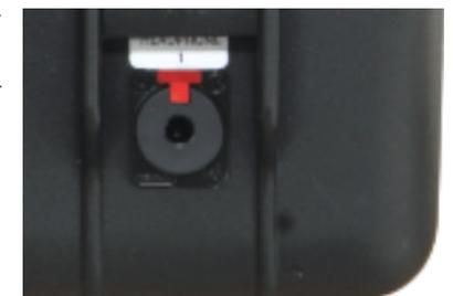
(Fig. 23) 6.35 mm headphone jack on the front of the case
