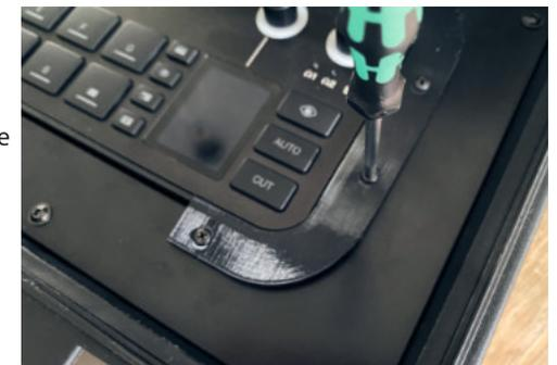
(Fig. 15) Screw C-Spanner into the 'Rodecaster Video case
