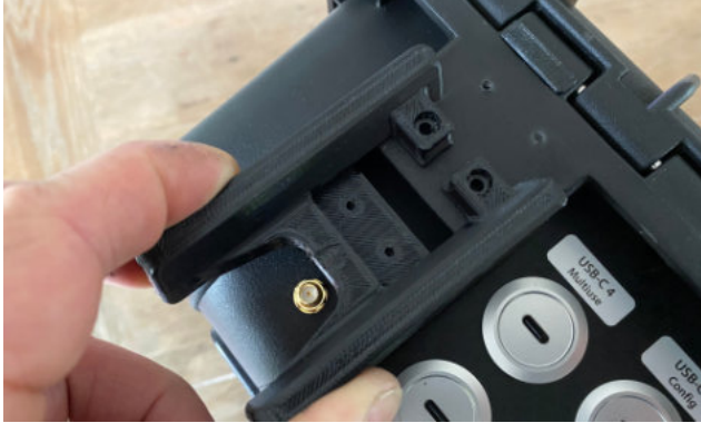
Inserting the antenna guard into the molded pocket on the back of the case
